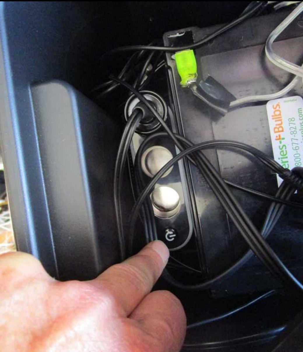
**Verify the Watec power plug is OFF: That means, lift the OccBox2 top layer and look at the triple-socket on the LEFT side (up against the wall as shown), and make sure it is not glowing purple. If it is, push button to power off.**
