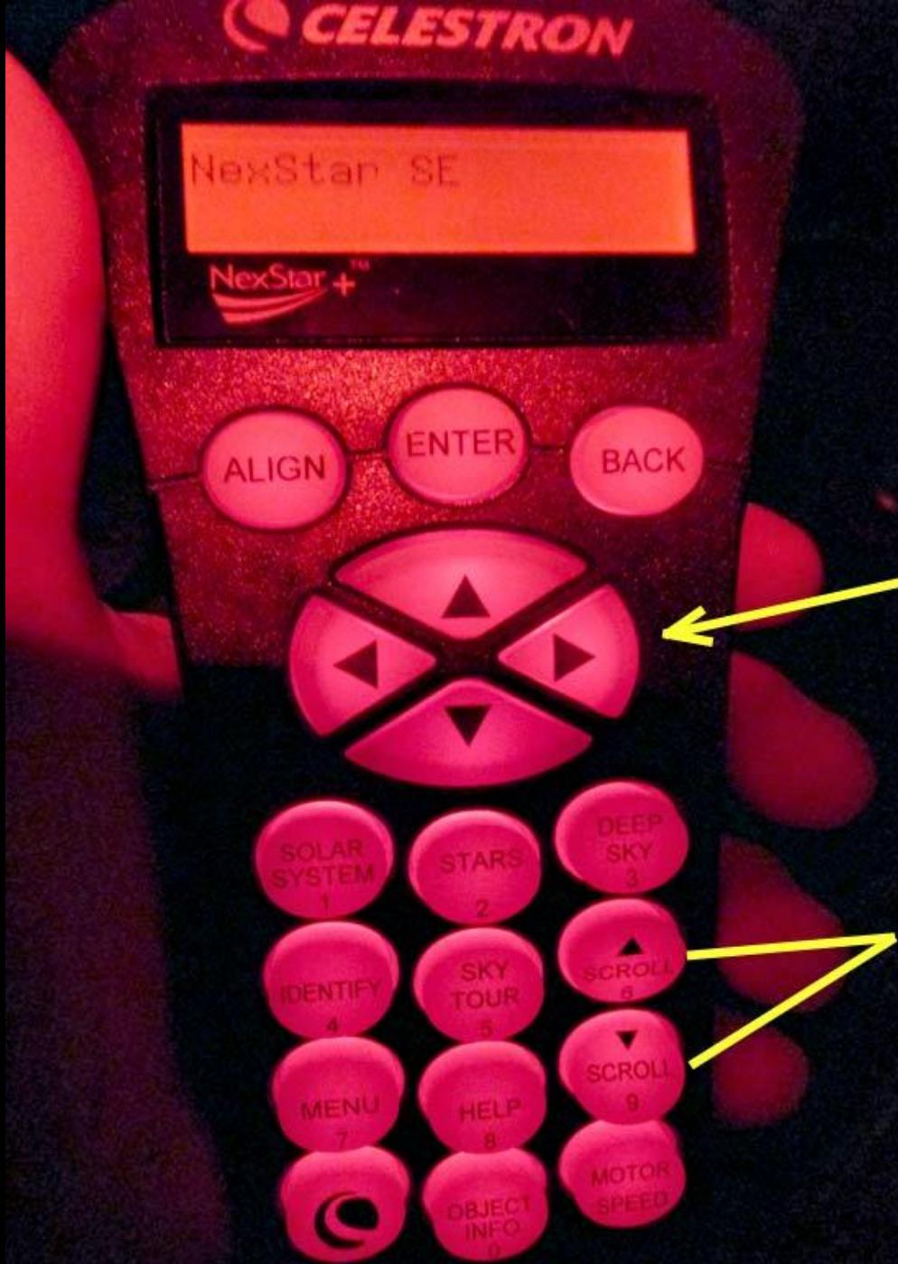
**Slew the scope up, down, left, and right**
