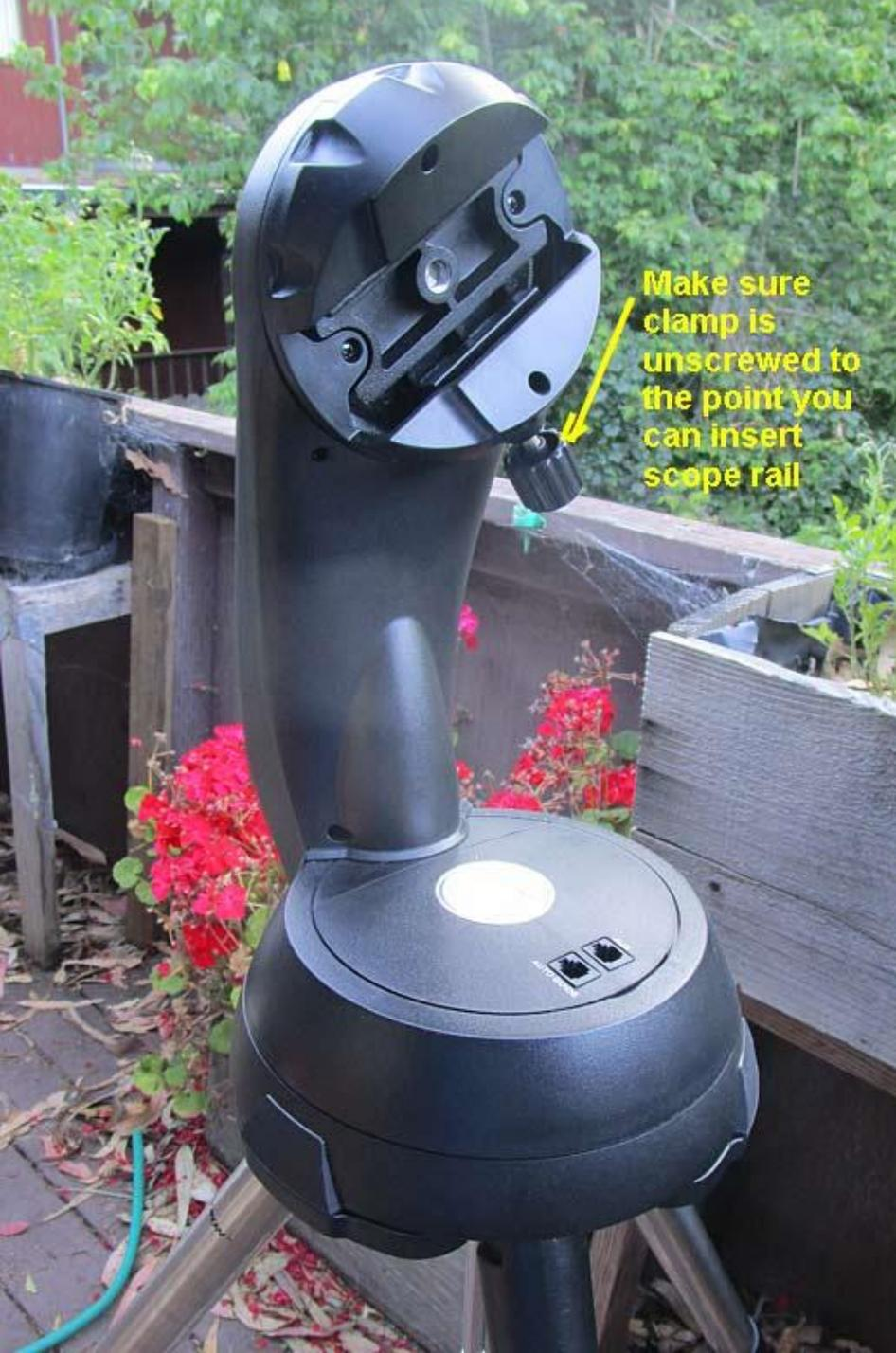
Make sure clamp is unscrewed to the point you can insert scope rail
