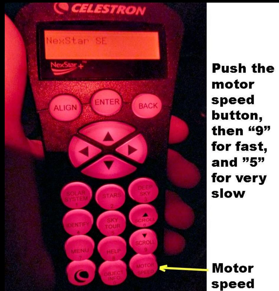
Push the motor speed button, then "9" for fast, and "5" for very slow
