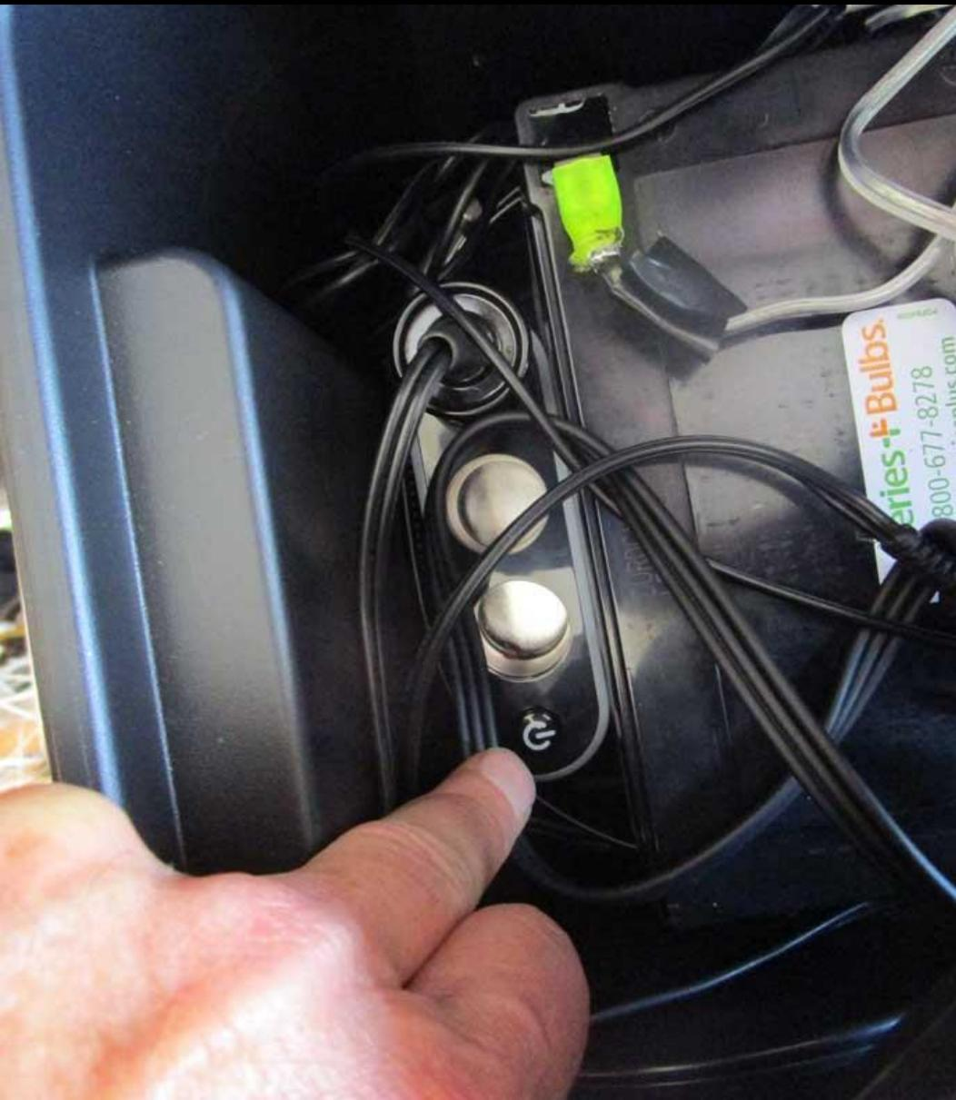
Lift the OccBox2 lid, and push the left triple-socket power button on, powering the Watec camera. Verify the triple socket rim glows purple. If not, you may have blown a fuse in the male 12VDC jack plugged into the triple socket at top. Replace fuse and try again.
