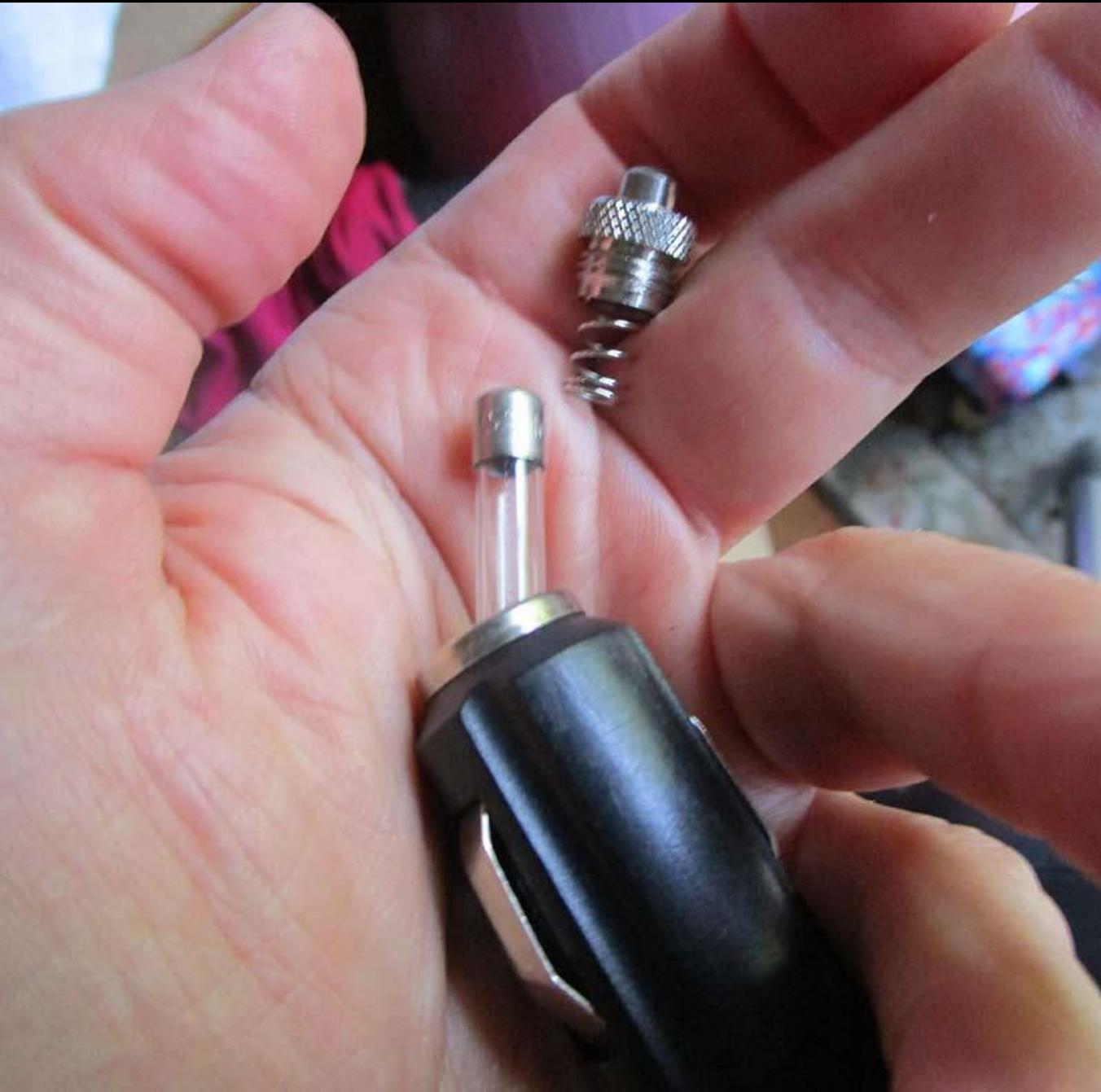
If it's the plug to the scope, unscrew the tip and check the fuse (glass fuse here). If it's a ceramic fuse you won't be able to tell if it's blown, so just try replacing it anyway. It takes the long 5 amp
