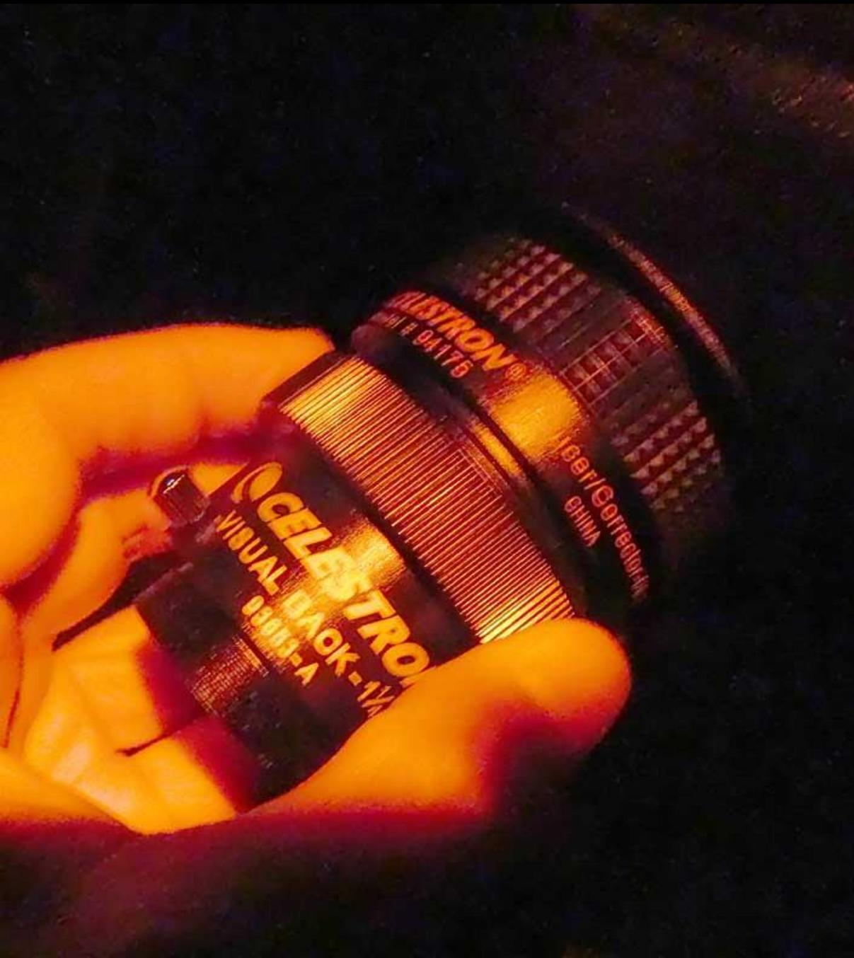
**Before mounting to the scope, screw the 1.25" Celestron visual back and f/3.3 reducer together. Then screw the f/3.3 threads onto the scope. FYI there is 35mm of separation from the lens surface of the f/3.3 reducer to the far tail end of the visual back.**
