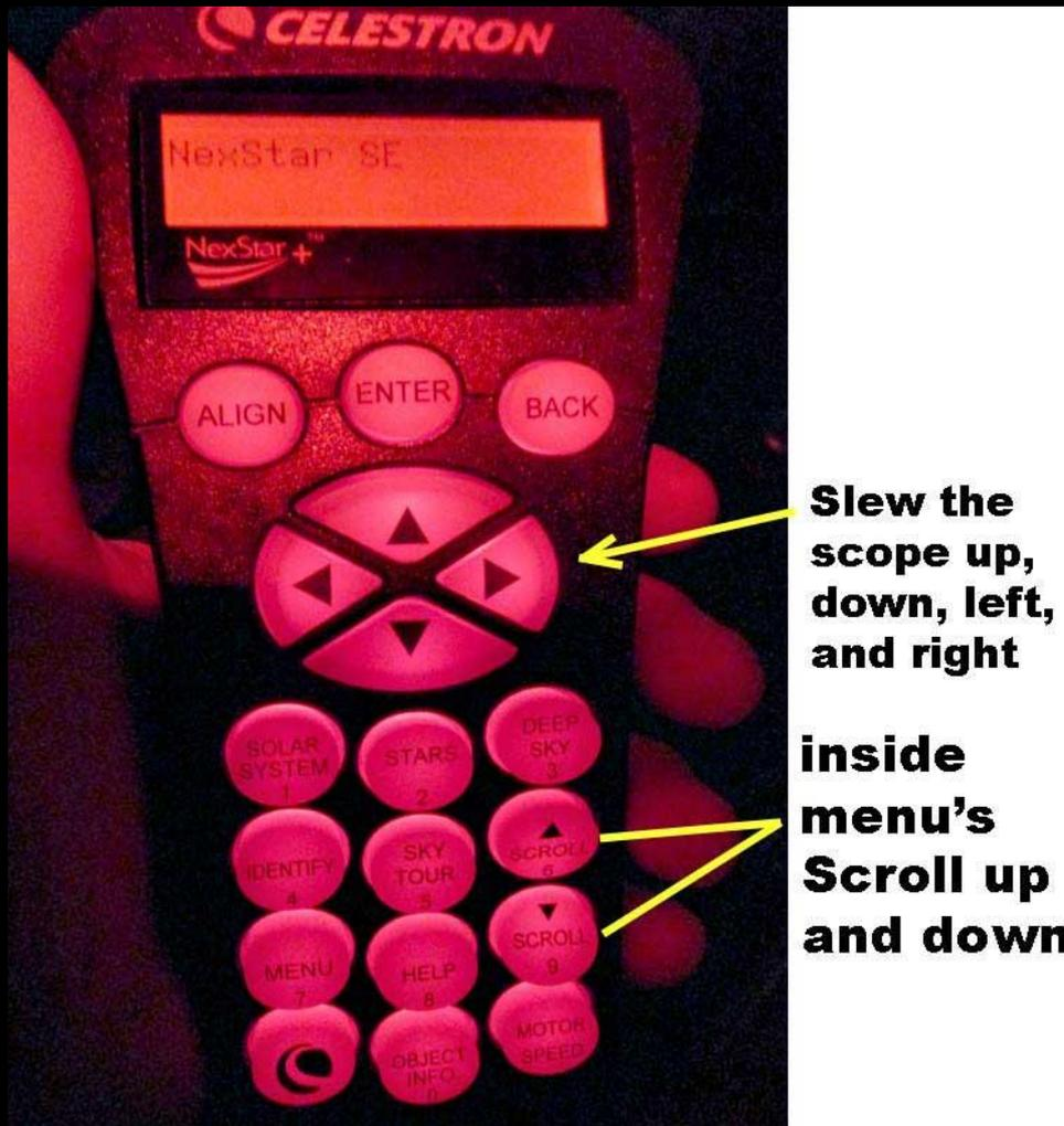
**Slew the scope up, down, left, and right**
